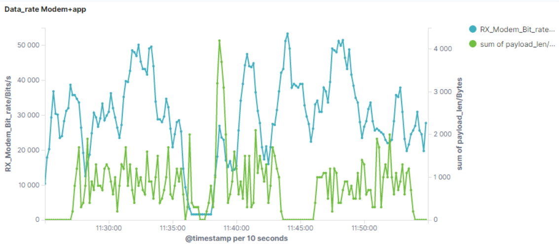
Figure 12: MODEM data-rate in bits/s averaged over 10 s (blue), and IP received throughput in bytes per 10 s (green) during phase C.
