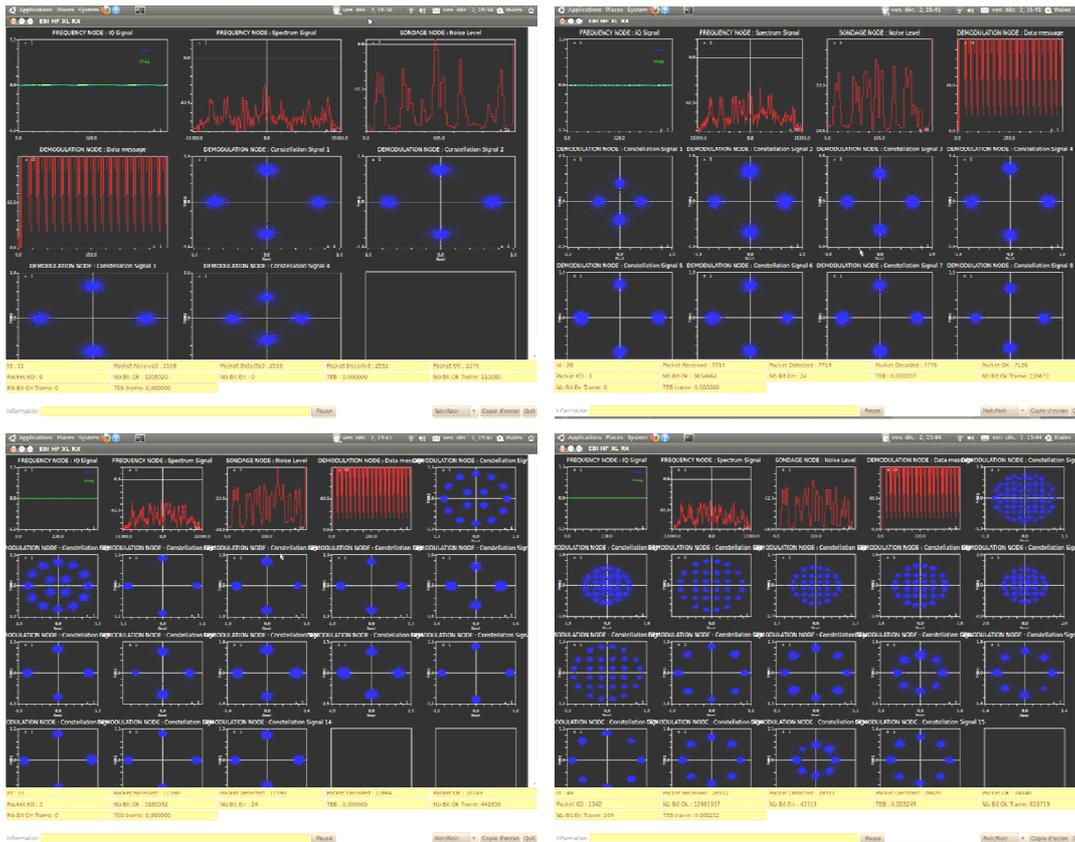
**Figure 7 – Automatic adaptation for the HF XL waveform: illustration of 4 different steps converging to a 92 kb/s link.**
