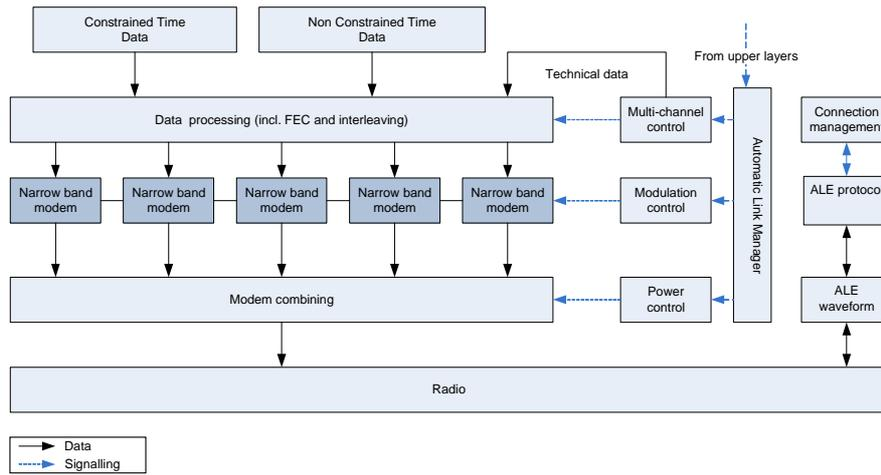
**Figure 3 – HF XL transmitter block diagram.**
