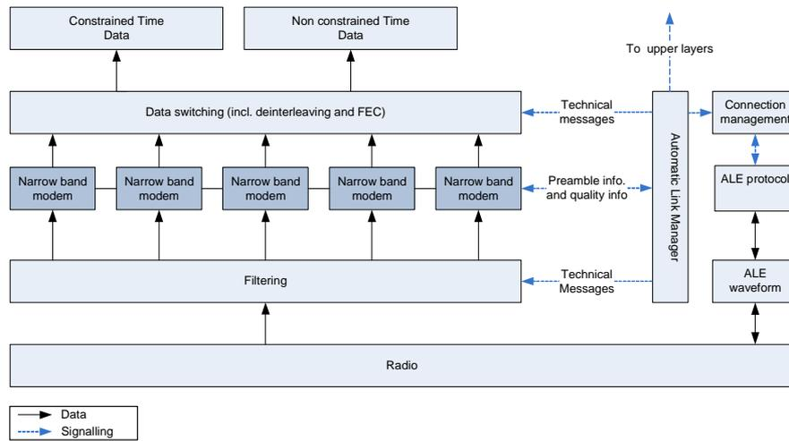
**Figure 4 – HF XL receiver block diagram.**
