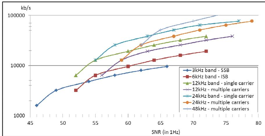
**Figure 1 – Comparing the required SNR for different contiguous and noncontiguous configurations.**
