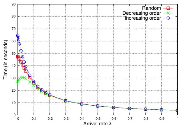
Fig. 6. ALE duration in function of the load, for different frequency selection strategies
