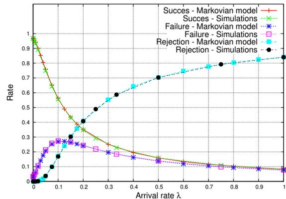
Fig. 4. ALE acceptance rate in function of the load, for  $p_s = 0.5$
