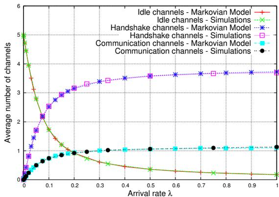
Fig. 3. State of channels in function of the load, for  $p_s = 0.5$
