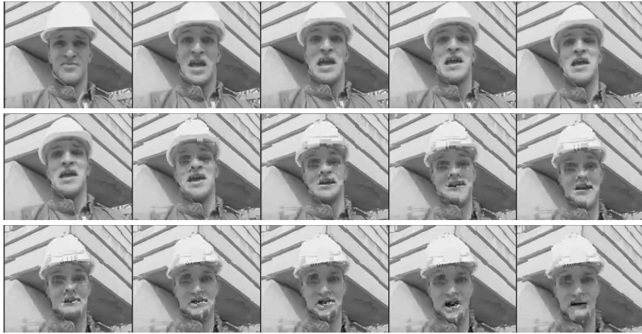
Fig. 20. Visual results over a GOP ( N=15 ) in an erroneous environment for the “Normal” configuration, Foreman sequence (6th frame impaired).
