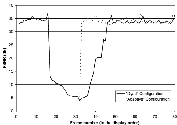
Fig. 23. 'Foreman' PSNR evolution comparison in noisy environment: "Dyad" configuration vs. "Adaptive" mode.
