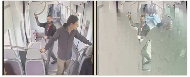
Fig. 3. Visual illustration of the video quality for dynamic protection rate driven by the Data Supervisor (left) and fixed protection rate (right) for BOSS ‘Anomaly’ sequence.
