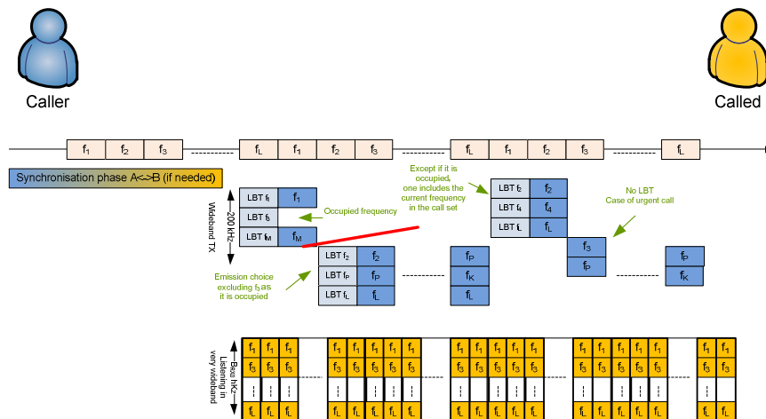
Figure 7: Illustration of the wideband ALE phase 2 including the wideband emission acceleration, with backward compatibility with an existing asynchronous ALE in the case of a very wideband receiver (synchronous mode).
